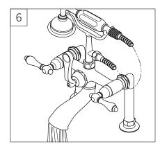
Turn on both hot and cold valves, let water run for at least one minute, this will clear any debris left in the line.
