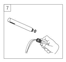
Remove shower by unscrewing the shower 'n a counter clockwise direction, turn on both hot and cold vahies and let water run for at least one minute, this will clear any debris left in the line.
