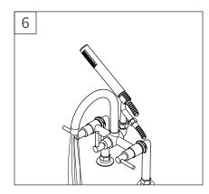
Turn on the faucet and let hot and cold water to run for a least one minute to clean any debris inside the water line.
