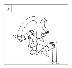
Place a washer between the s'de hole of the shower cradle and the cone nut of the shower hose. Tighten the cone nut.
