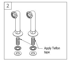
Apply Teflon tape on the threads of the copper shank. Install the risers.
