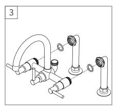
Before mounting the faucet onto supply risers, apply small black washers onto both water inlets of faucet.
