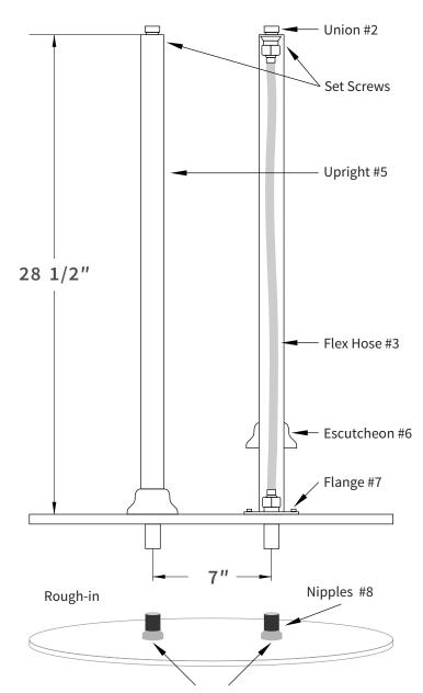
Install 11/2-14 NPS pipe nipples protruding 1" above finished floor
